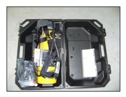
Each swabbing rig is equipped with two 30 min self-contained breathing apparatus. Swab Master Ltd. uses the Scott 2.2 self-contained breathing apparatus shown here.
